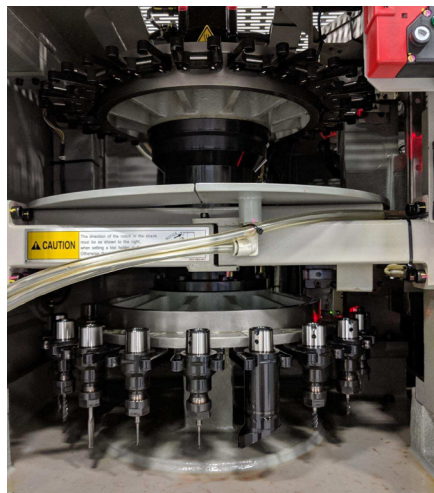
SS38MH-5AX Tool Magazine
