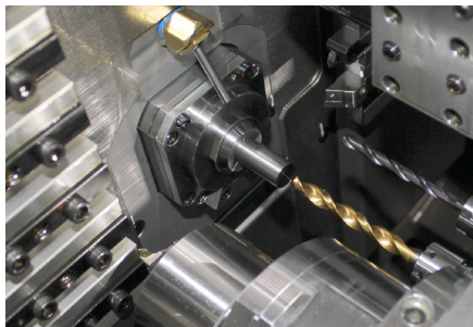
Deep Hole Drilling
