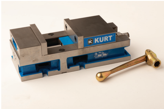
Vise 6" Kurt vise and mounting hardware - model DX6. Opens to 9".
