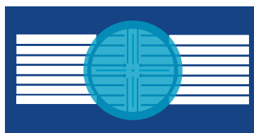
Integrated rotary milling | turning table (located in the center of the table)
