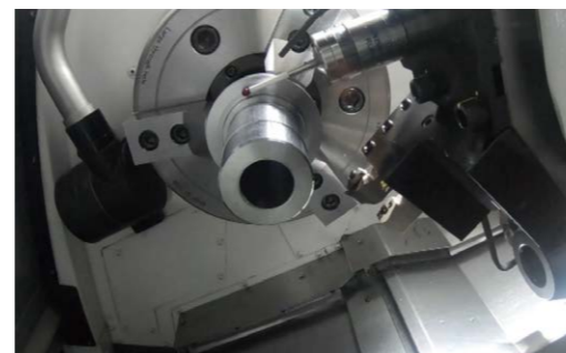
This photo shows measurements taken along the Y-axis by an LB3000 EX III with Y-axis specs.
