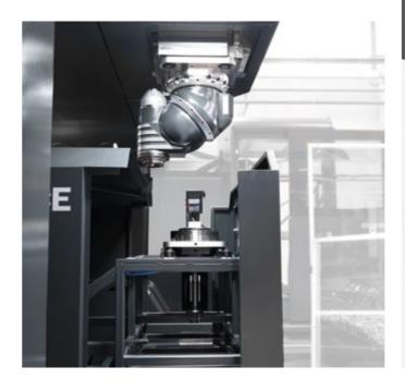
High torque direct drive spindle motor inside the ram, with a built-in cooling system.
