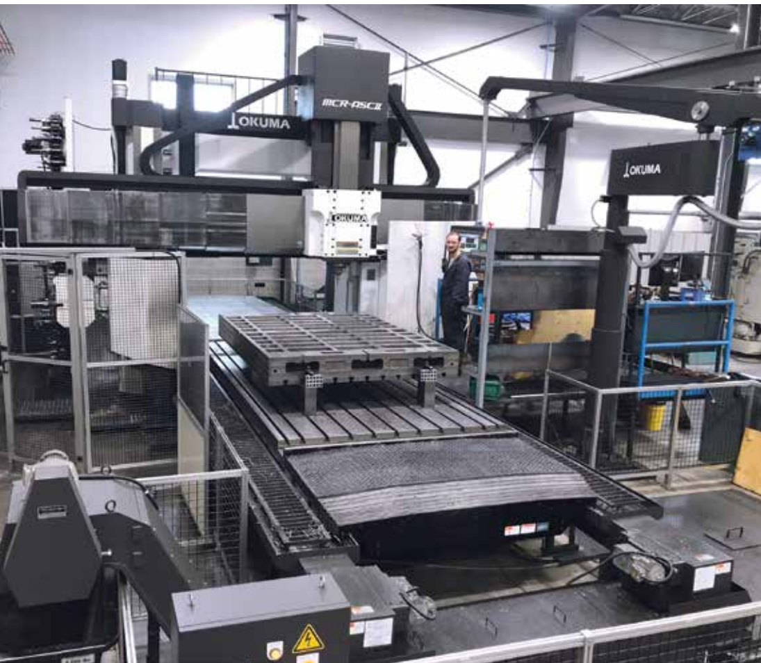
The MCR-A5CII from Okuma plays a key role in XL Tool's large part machining operations. XL TOOL
