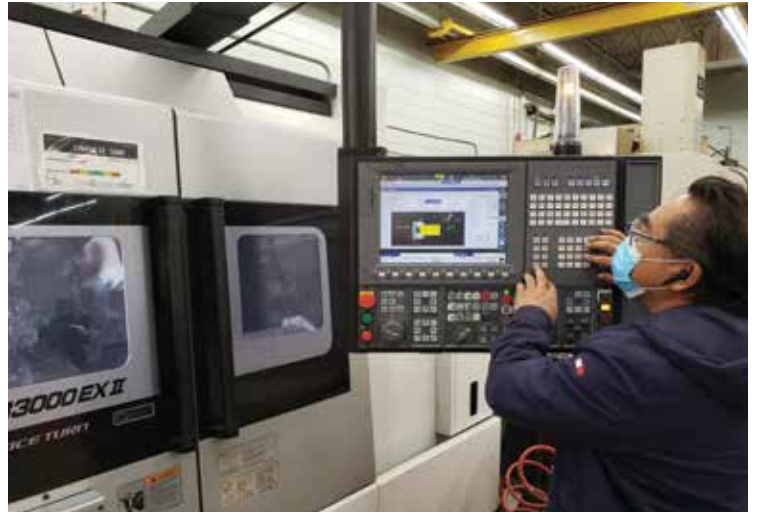
The Okuma machine is perfect for small parts, especially ones with low weights. Most of the shop’s other machines produce 18- to 42-in.-dia. parts, while the Okuma machine is used to produce its 10-in.-dia family of tensiometers.
